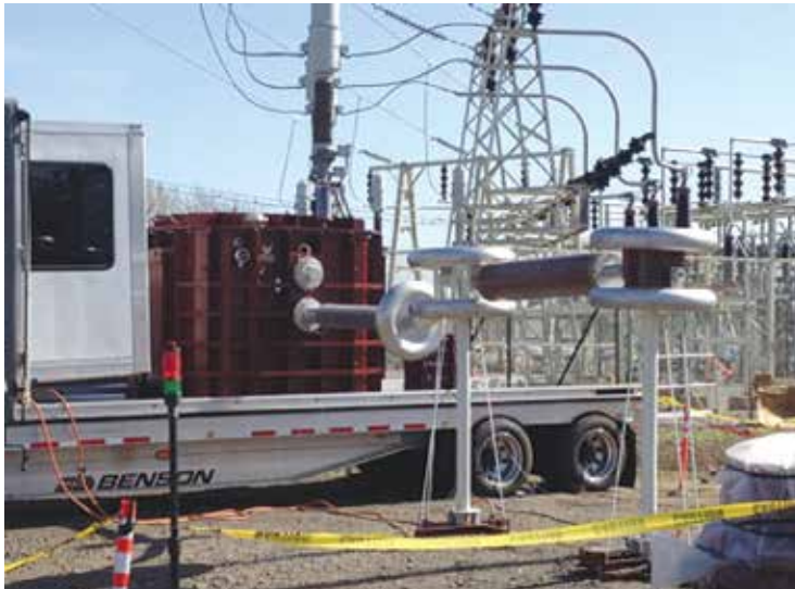
Dielectric testing 138 KV class transmission cable in Long Island, NY.
