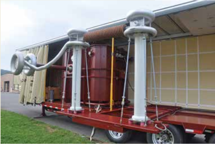
VRTS Trailer 16 MVA, 225 kV, f = 25...300 Hz
