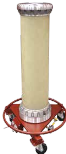
100 kV SF 6 Gas Insulated Standard Capacitor and tan \delta -bridge
