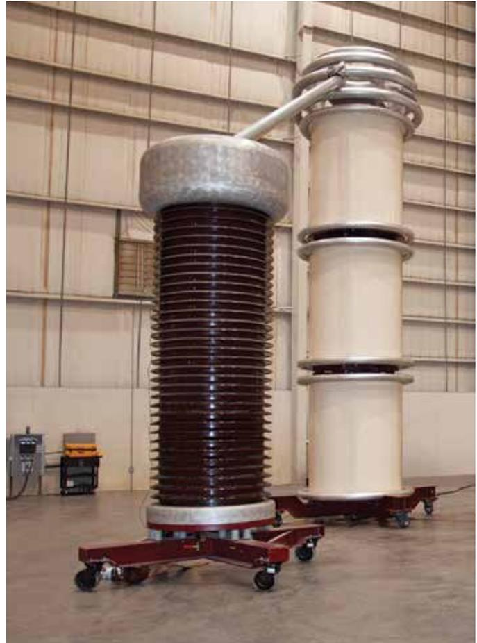
800 kV SF6 Gas Insulated Standard Capacitor and
